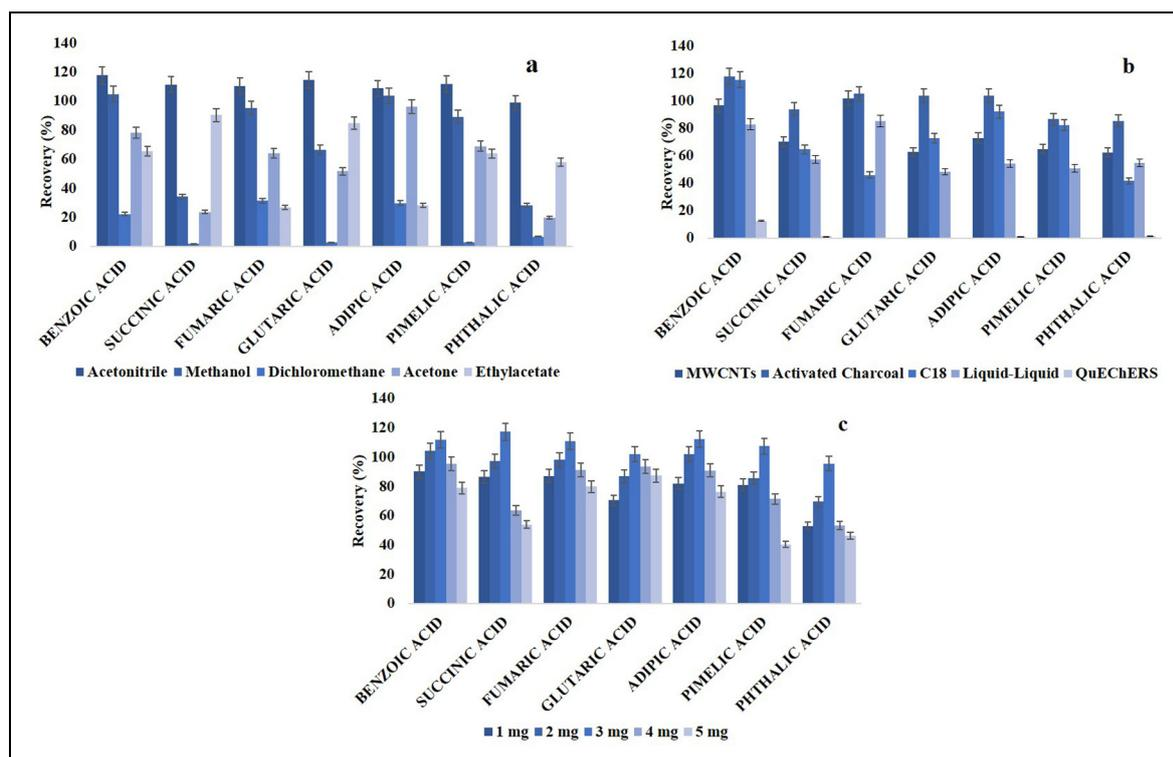
**Figure 2.** Recovery of the analytes at a concentration of 10 ng/g **a**, different extraction solvents; **b**, different cleanup methods; and **c**, amount of activated charcoal.
