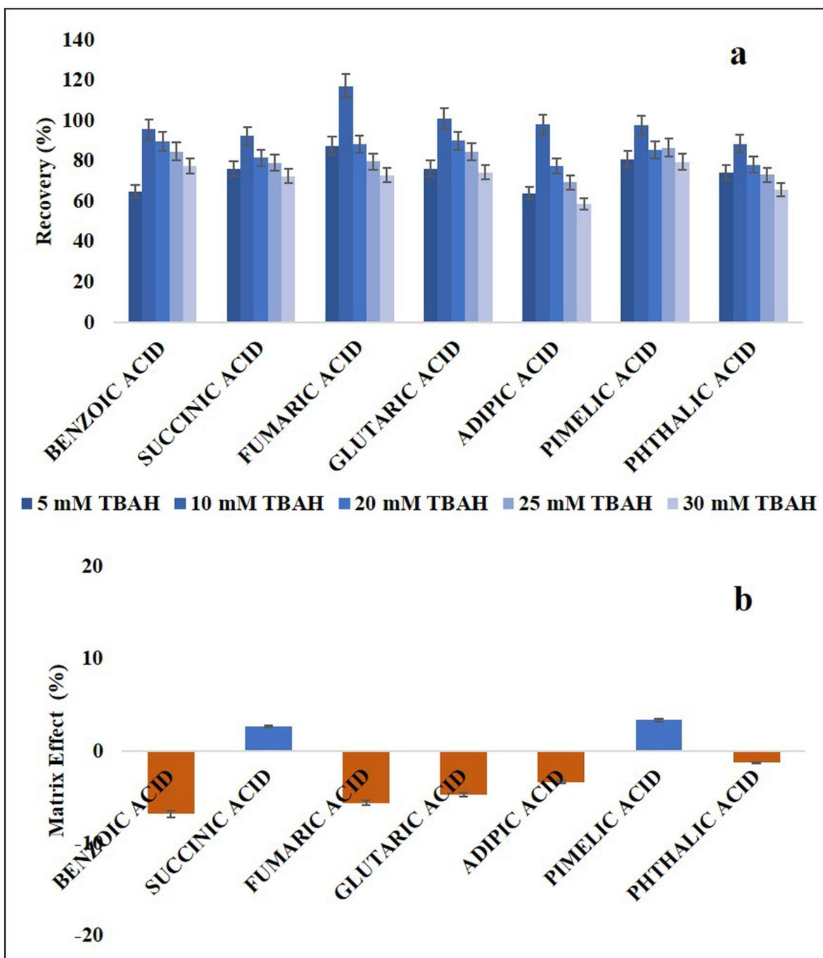
**Figure 3.** Recovery of the analytes at a concentration of 10 ng/g **a**, TBAH with different concentrations; and **b**, matrix effects.
