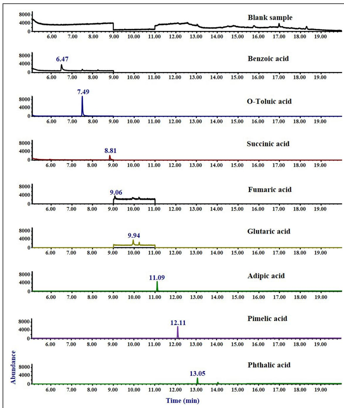
**Figure 1.** GC-MS extracted ion chromatograms of organic acids obtained from the fortified fish feed at LLOQ level.
